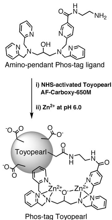
**Figure 1.** Preparation of Phos-tag Toyopearl, the novel Zn(II)-IMAC bead, by using a Phos-tag derivative having a 2-aminoethylcarbamoyl group (amino-pendant Phos-tag) and NHS-activated Toyopearl AF-Carboxy-650M gel.
