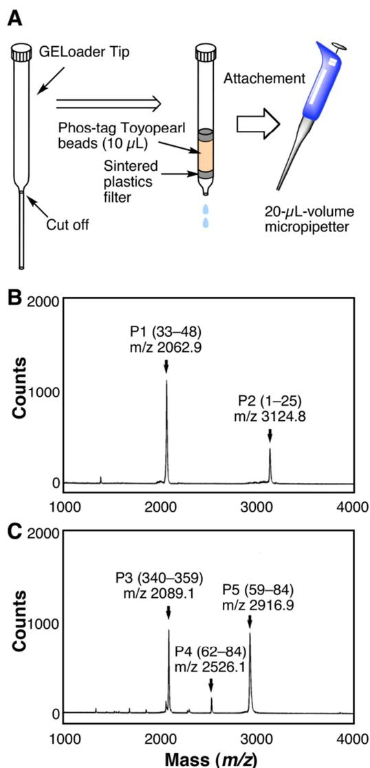
**Figure 4.** Affinity pipette microtip column chromatography for the separation of phosphopeptides. Scheme for the preparation of the pipette microtip column packed with Phos-tag Toyopearl (Phos-tag tip) (A). MALDI-TOF/MS analysis of each elution fraction after the affinity pipette microtip column chromatographic separation of the tryptic digest of  $\beta$ -casein (B) and in-gel tryptic digest of ovalbumin (C) as samples.
