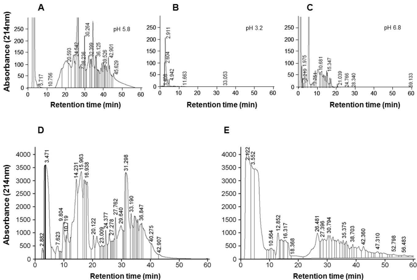
**Figure 2.** Representative HILIC and SCX chromatograms. (A-C) HILIC chromatograms of 100 pmol BSA digest separated using solvents of different pH values. (D) HILIC chromatogram of guard cell protein digest. (E) SCX chromatogram of guard cell protein digest.
